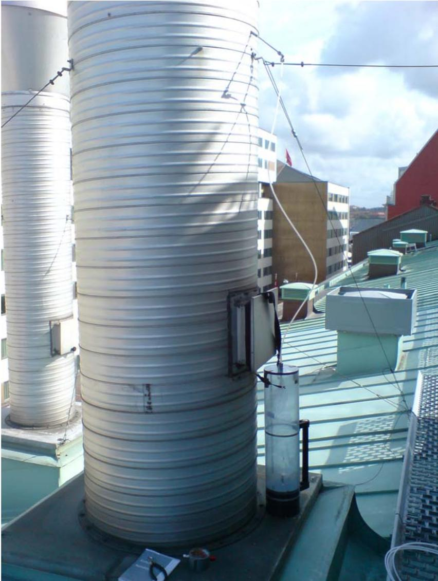
Figure 1 Odour sampling after the fan unit.
