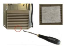
2. Remove the front of the filter with a screwdriver. If the filter is dirty, it should be replaced.
